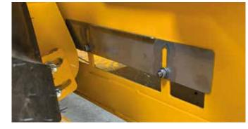
To optimize bottom fans efficiency **GT3** is equipped with **MAXflow** system. 2 trapdoors located each side of main conveyor, underneath bottom fans, adjusts air intake to fans for an optimum MOG extraction. Trapdoor position
